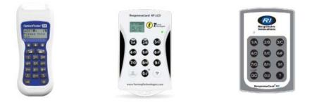
The exact layout of the device depends on the specific system, but they usually include several input buttons, and often a screen or LEDs to provide feedback to the voter. In considering handset options, the committee will require a device containing a screen that provides positive confirmation to the user that the vote was properly sent and recorded.
